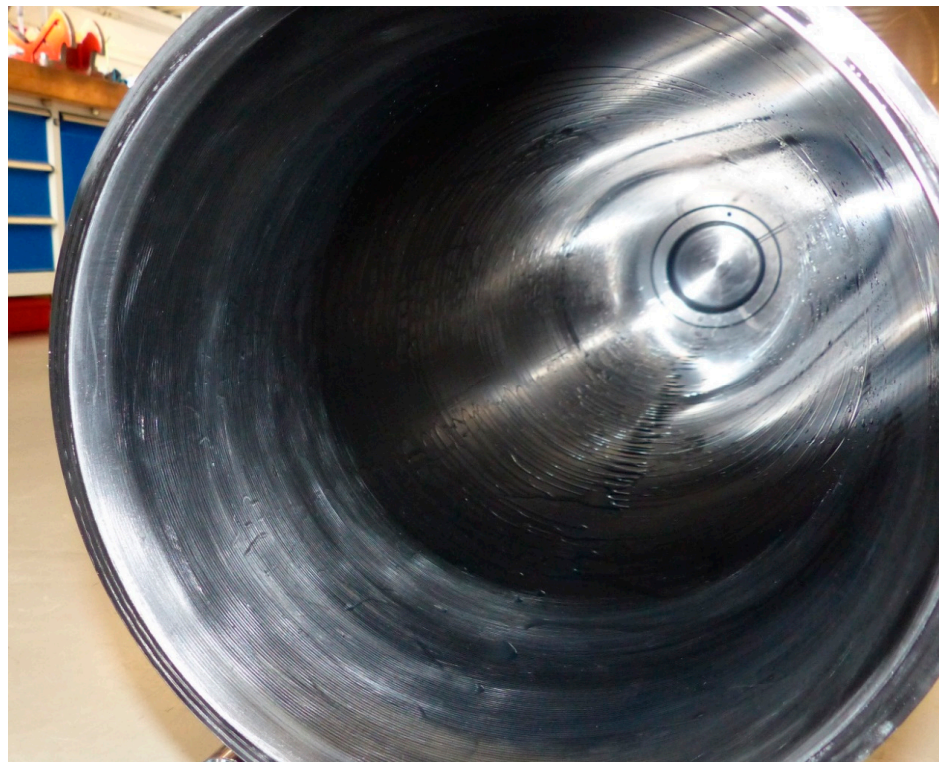
Figure 9. A prototype of a CFRP piston accumulator with a steel liner on the inner surface of the CFRP tube.
